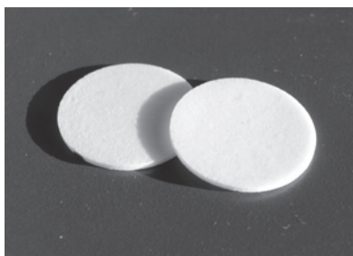
Figure 4.3: Photos of compressed solid acid discs ( \varnothing 10 mm, 1 mm thick)
