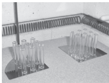
Figure 5.3. Fusion bonding of a batch of glass tubes of 30 mm length onto silicon wafer
